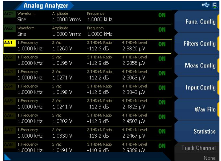
Figure 4. The U8903B's GUI, showing 8 analyzer channel measurements.
