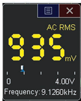
Figure 24: DVM 3-digit voltage and 5-digit frequency measurements always at your fingertips.
