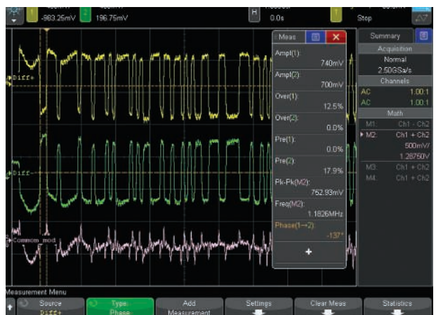
Figure 23: Dual channel WaveGen output of differential arbitrary signals. Common mode is shown as a math function.
