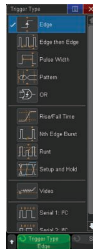
Figure 42: Wide array of advanced parametric trigger modes.
