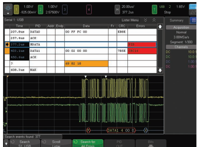
Figure 20: USB 2.0 trigger, decode and “lister” display.
