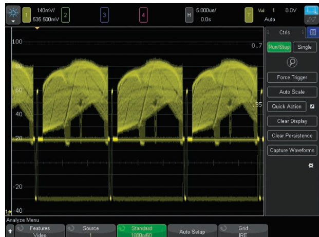
Figure 26: Triggering on 1080p HDTV signal analysis.
