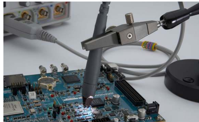
Figure 34: The N2750A InfiniiMode probe allows convenient measurement of differential, single-ended, and common mode signals with a single probe tip without reconnecting the probe to change the connection.
