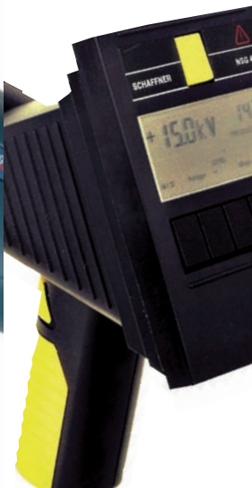
NSG 435 ESD generator up to 15kV
