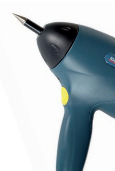
NSG 438 ESD generator up to 30kV
