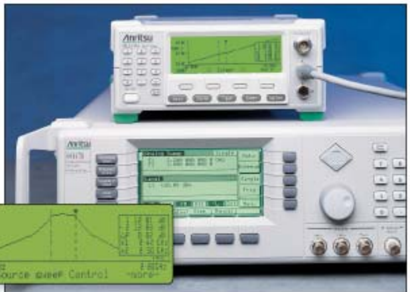
Source Sweep Graphic Display. Acquire power sweep or frequency sweep data at speeds greater than fifteen sweeps per second ( GPIB to PC screen update rate). The meter automatically generates sweep synchronization with Anritsu 68000B or 69000A series Synthesized Sweep Generators.
