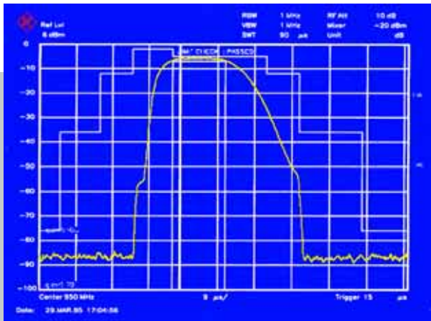
5 GAP SWEEP: simultaneous measurement of pulse rise and fall time with high time resolution
