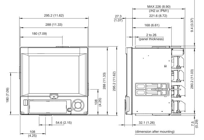
Note: If not specified, the tolerance is  $\pm$ 3%. However, for dimentions less than 10mm, the tolerance is  $\pm$ 0.3mm.
