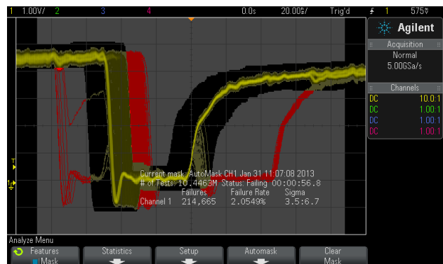
Limit testing made easy with the "automask" feature
